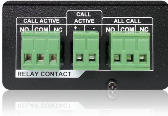
EMPR-8007 provided 2 relay contact for trigger other customize device. However, at the middle of the diagram external trigger port is provided (CALL ACTIVE +/-) for other emergency panel to trigger the current system into emergency mode.
