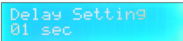
*Figure 1.6.5: Minimum value of Delay Setting – 1 second.*
